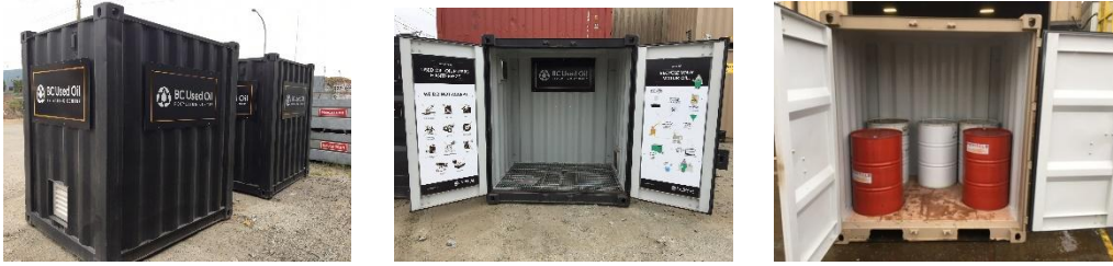
Examples of 8 ft HC seacan 7 ft (w) x 6.5 ft (l) x 8 ft (h) with 420 litres secondary spill containment
